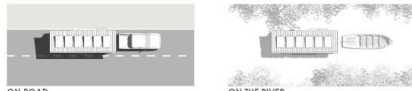
ON ROAD ON THE RIVER The modularity has been planned to allow transportation by a trailer on conventional roads.
