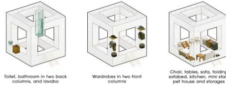
Toilet, bathroom in two back columns, and lavabo Wardrobes in two front columns Chair, tables, sofa, folding sofa-bed, kitchen, mini stairs, pet house and storages
