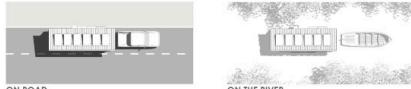
ON ROAD ON THE RIVER The modularity has been planned to allow transportation by a trailer on conventional roads.
