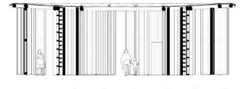
Section showing outer circulation corridor and internal community courtyard
